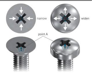
Cross recess is easily deformed when forming screws. Countersunk screw: cross entrance may become narrow Pan head screw: cross entrance may widen
